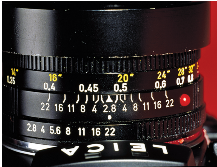
Fig. 3 The aperture on a macro lens should not be set smaller than f22 to prevent diffraction
