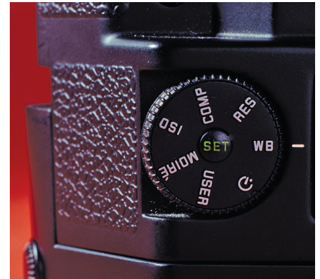
Fig. 20 WB (white balance) setting dial on a digital camera back
