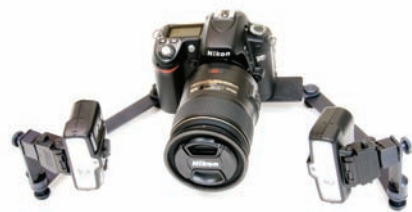
Figure 1 Nikon D90 camera with the Nikon R1C1 dual-point flash and Winphotec Bracket.
