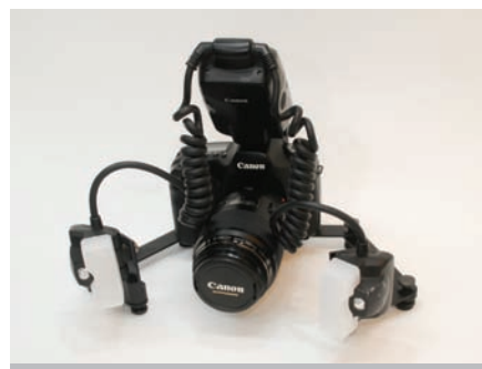
Figure 2 Canon SX1 camera with the Canon 24 EX dual-point flash and Winphotec Bracket.
